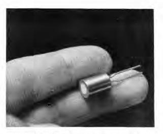
HIGH TEMPERATURE resistant exploding bridge wire detonator invented by Bill Leslie (1915).
